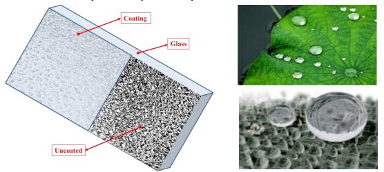
The application fields of Easy-cleaning Glass: curtain wall glass for buildings, solar photovoltaic glass, shower room glass, rear view mirrors for cars, greenhouse glass, and so on.
